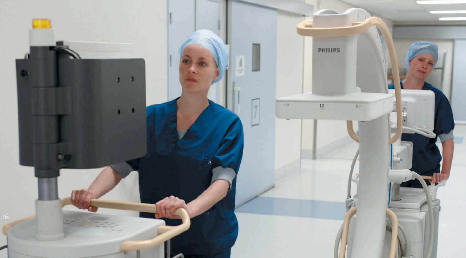
For easy and safe transport and storage, simply fold the monitors and move them to their lowest position.
