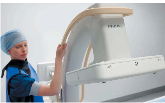
The same reference numbers are clearly visible on the clinical image and on the Flat Detector (ClearGuide) so everyone knows which direction is meant when positioning the C-arm.
